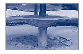
adhesive anchors used in concrete. This type of concrete anchor is recognized as an important structural connection in many applications, and the design, use, and installation procedures are intertwined to ensure proper performance. It's important to note that adhesive anchor installer certification will be required when the 2011 ACI
